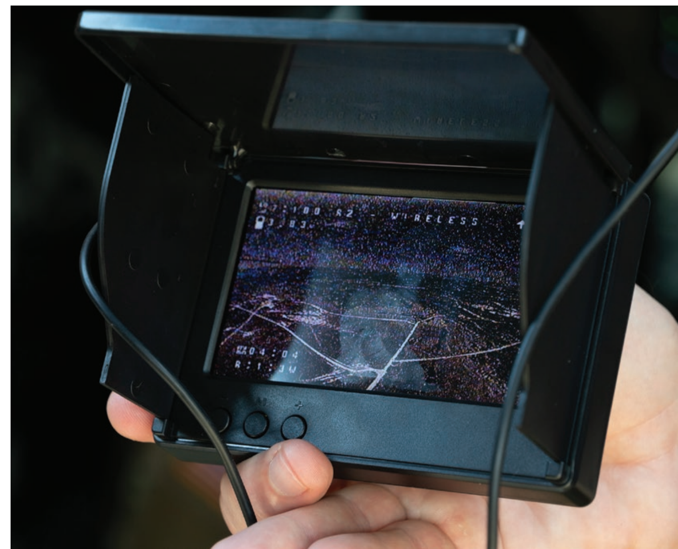
A passive drone detection device hijacks the footage of a small unmanned aircraft system during Operation Return of the Condor on Fort Hood, Texas, Aug. 25, 2025. Operation Return of the Condor served as a testing ground for drone detection and counter sUAS tactics by bringing together First Team Troopers and industry partners for experimentation and innovation. (U.S. Army photo by Spc. Julian Winston)
