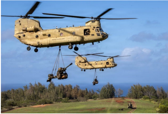
Two Chinook Helicopters sling load M119 Howitzers during an air assault operation (U.S. Army photo by Sgt. Olivia Cowart)
