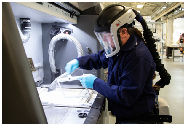
An additive manufacturing specialist at Rock-Island Arsenal- Joint Manufacturing Technology Center brushing powder off completed ventilator housing parts
