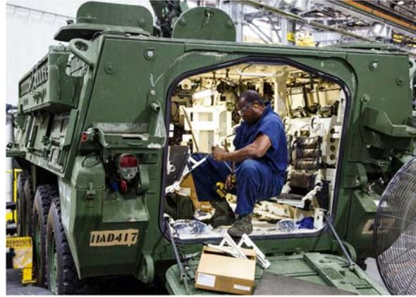
An Anniston Army Depot employee works on installing new internal parts on a Stryker.
