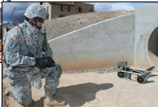
Searching culvert with Small Unmanned Ground Vehicle
