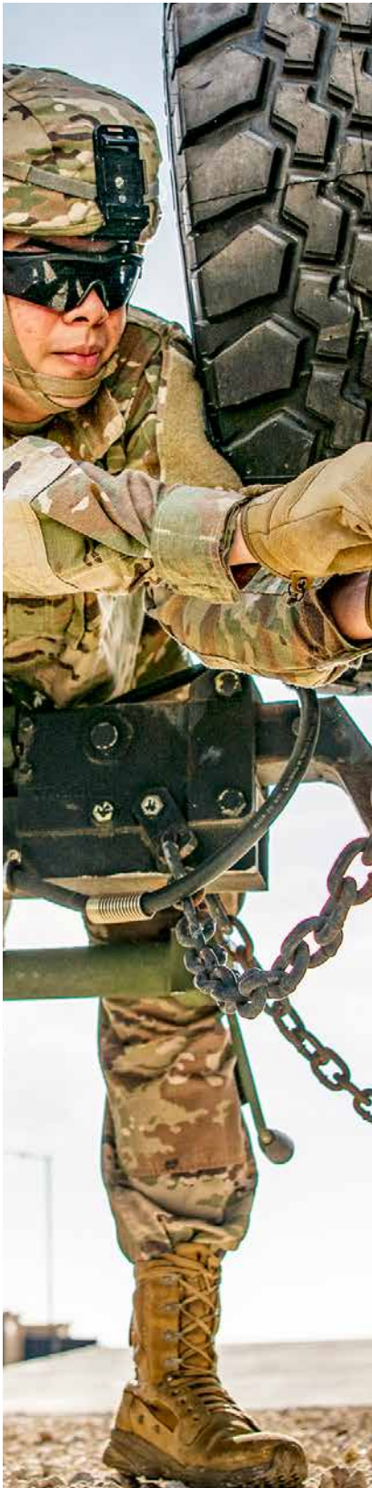
Securing a trailer to the back of a Humvee (U.S. Army photo by Sgt. Dustin D. Biven)
